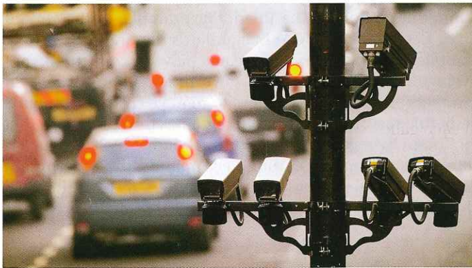
Big Brother Is Watching Your Car! Closed circuit television cameras loom above traffic in central London to monitor the license plates of the estimated 250,000 cars entering the city each day. Drivers pay a “congestion charge” to drive in central London, making it more expensive to drive there, with the ultimate goal of reducing traffic backups.
